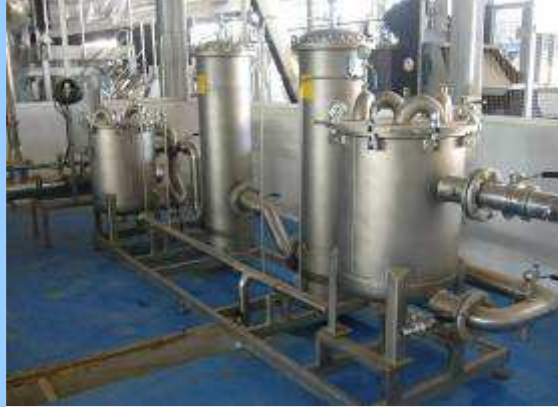
Filtration platform 25 down to 1 micron ( \mu ), 80 m 3 /h
