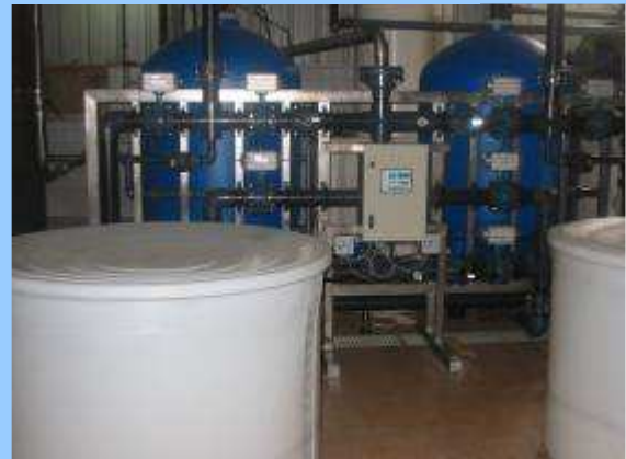
Nitrate removal units with selected ion exchanges resin, 25 and 55 m 3 /h
